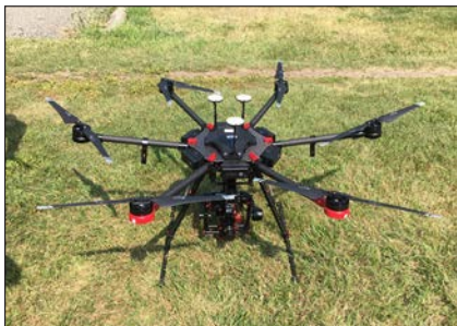
Drone with hyperspectral imaging systems ready to collect data. Photo by Joseph Shaw.
