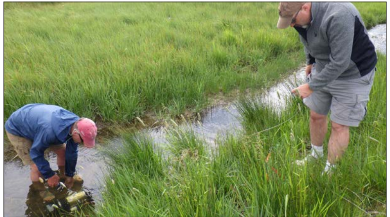
Mike DeGrandpre and Cory Beatty deploy a stream sensor array (measuring continuous dissolved oxygen, carbon dioxide, nitrate, and more) in Louse Creek, a headwater tributary of the Judith River. Photo by Stephanie Ewing.
