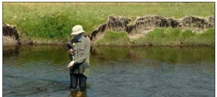
An undergraduate student researcher uses an electrical conductivity probe to measure water quality on the Upper Clark Fork River. Photo by Robert Payn.
